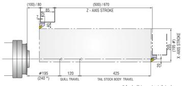
\* for built in center tailstock # for 12 station turret - (Short Stroke)
