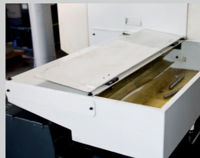
Long work piece ejection system
